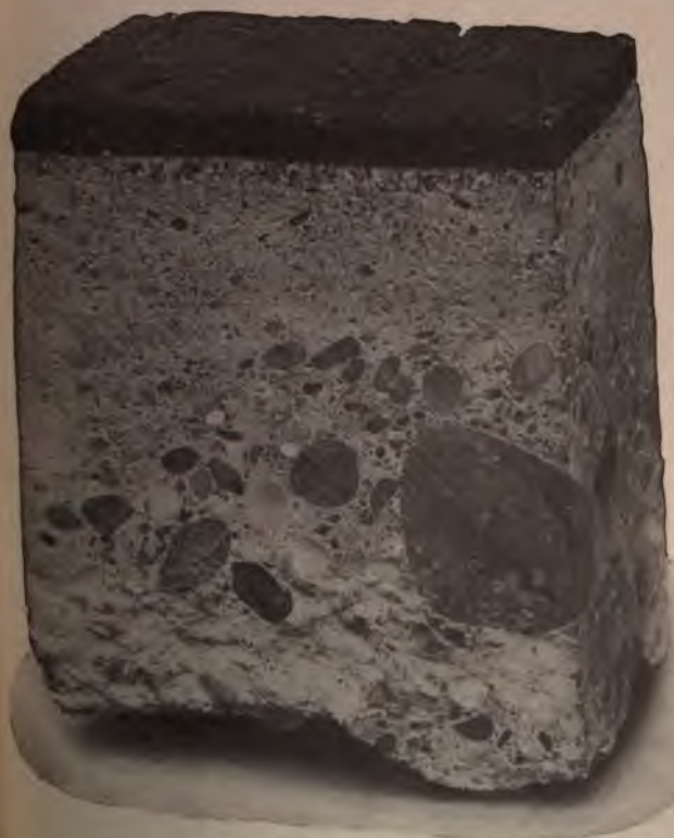
Section Cut from Dolarway Pavement.
